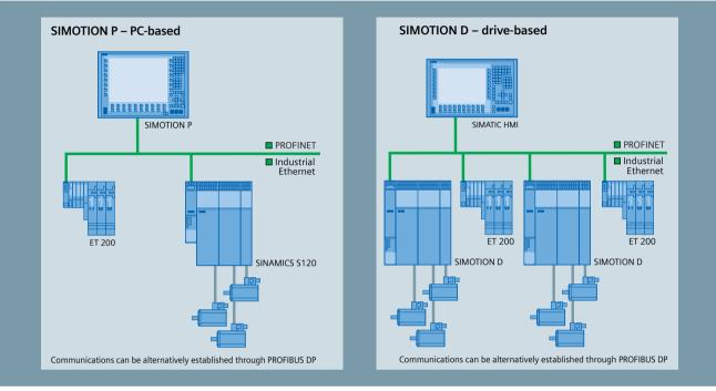
Solutions can also be implemented with SIMOTION D directly embedded in the drive. SIMOTION systems and servo drives are synchronized via PROFIBUS DP or PROFINET with PROFIdrive.
