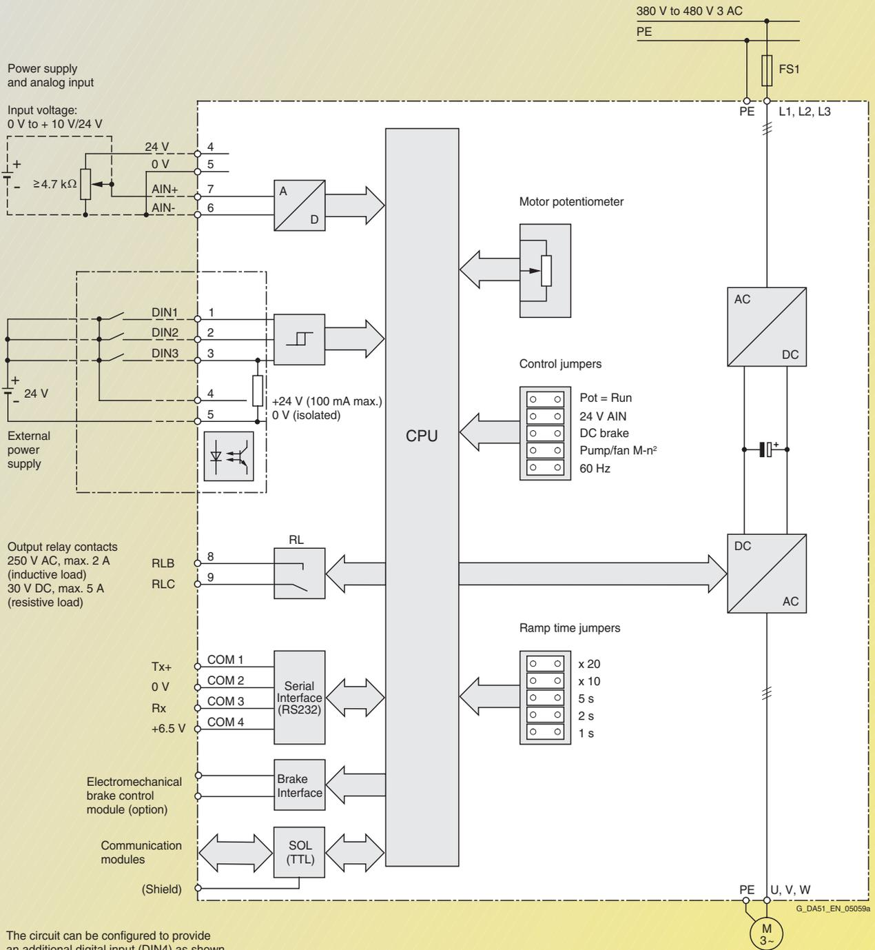
The circuit can be configured to provide an additional digital input (DIN4) as shown. Switching voltages must be greater than 4 V.
