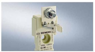
Flat terminals with screws are suitable for connecting busbars or cable lugs. They have a torsion-proof screw connection with shim, spring washer and nut. When tightening the nut, always ensure compliance with the specified torque due to the considerable leverage effect.
