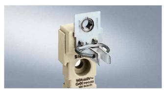
In the case of flat terminal with nut, connection of the nut to the terminal lug is torsion-proof. When tightening the nut, the torque must be observed because of the considerable leverage effect.
