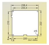
Fig. 2/2 Support plate, overall height approx. 72 mm
